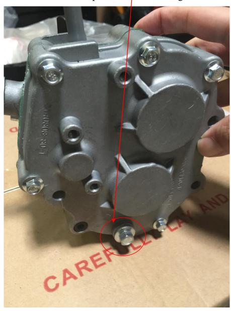
2. Close the drain plug when all the gear oil has been drained out, use hand to open the oil refill cap as indicated in the picture:
