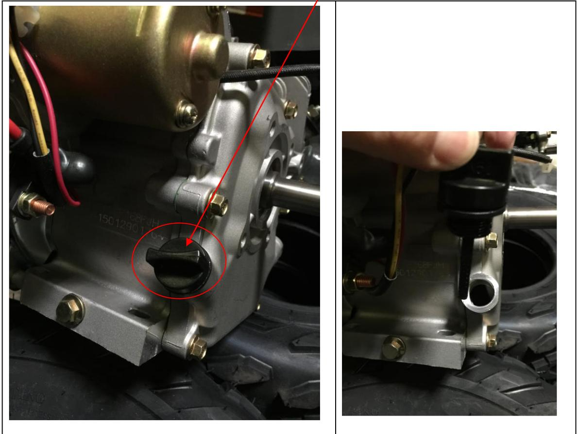
3. Refill engine oil SAE 10W-40 (Note: only engine oil for GASOLINE engine can be used!) 1 to 1.25 pint into the engine through the oil gage hole. Check the oil level on the oil gage stick to make sure the oil level inside the engine is correct.
