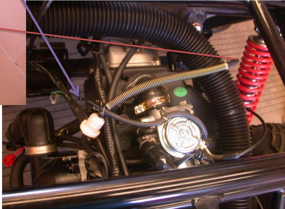
Connect the fuel line with the fuel tank
