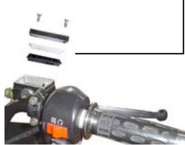
Fig. 7, Opening the Reservoir
