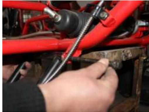
Put down the front up swing arm and screw off the bolts at the end of the arm. Take it to the fixture in the front of the **brake hub** and screw on tightly.
