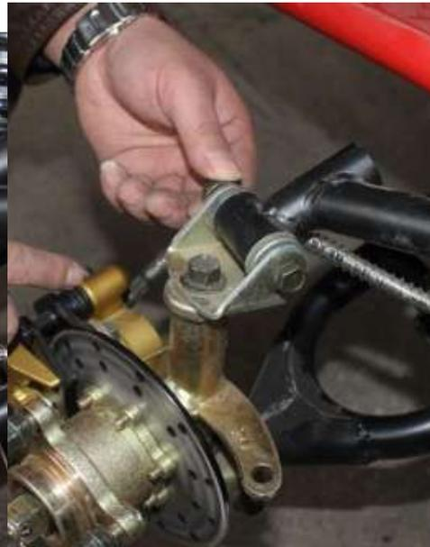
Now please check such rod for the steering. Screw on this rod to the end screw of the steering machine and make the nuts closed to the machines. For the another end please take off the pin and nuts first. When you screw the ball to the rod take it into the hole of the brake hub and screw on with such nut and pin.
