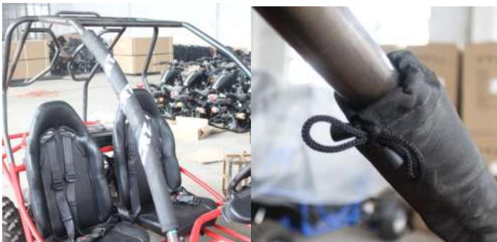
Now we got it. Our buggy is assembled. DO NOT in a hurry for racing. Please check once more all the bolts are screw up well and the fuel switch, the battery, the air press for tires. Then please check with our use's manual for your use and maintains.
