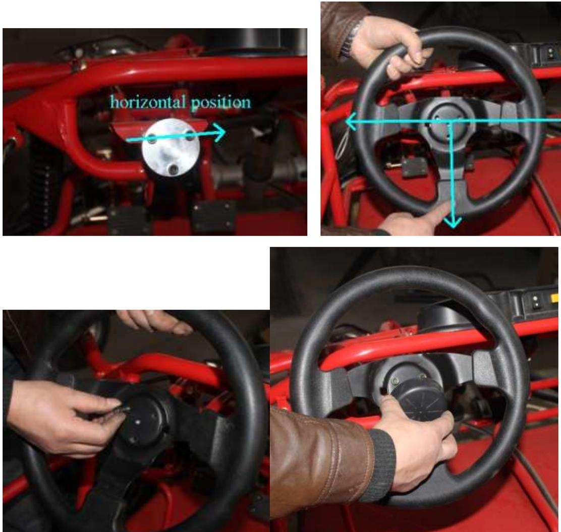
Let's make the wheel horizontal and check the front wheels. If it is **not in parallelism with the buggy median** we could take the rod round to make the wheels forward. Remember take the nuts close to the rod.
