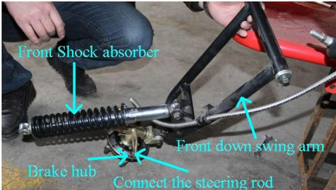
Screw off the long hex bolts of the Front down swing arm with the metal dust cover to the welding downside of the chassis. Fasten the arm to the frame tightly.
