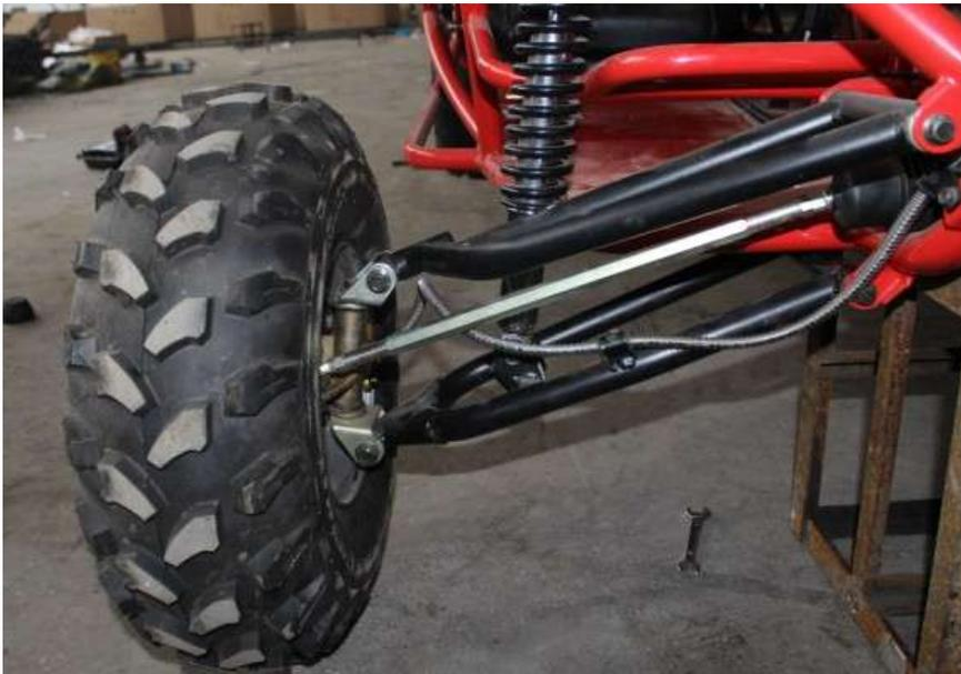
8. Now we could have the buggy on land already. Then we come to the steering wheel. Make sure the axis with a round plate welded is in the right position that is two wheel front in horizontal standard. Screw off the bolts and fix the steering wheel in the
