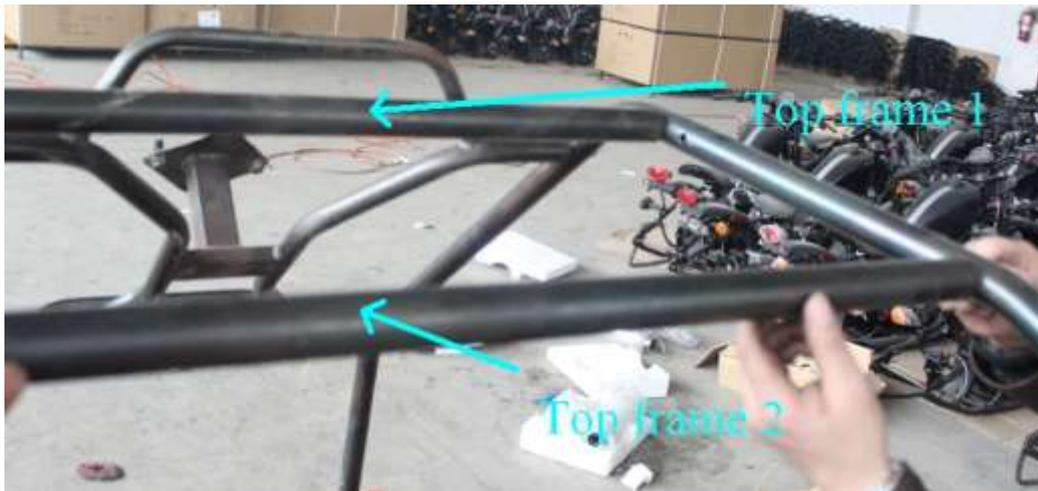
The last one is the middle frame from the back of the seat to the top frame. You could have them tightened in a same way.
