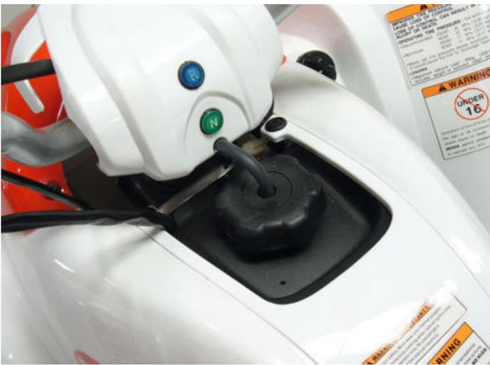
step18-fig2-Fuel cap vent hose routing
