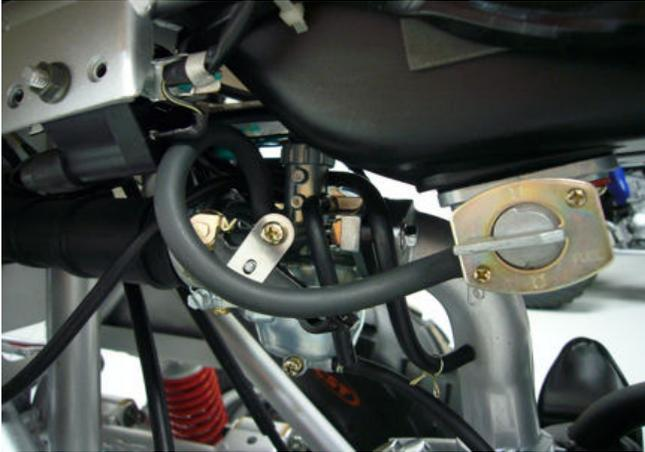
step10-fig1-Fuel line routing
