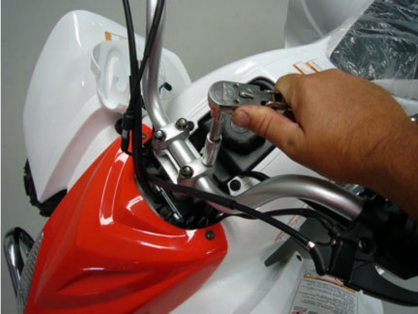
step08-fig1-Tighten handle bar bolts
