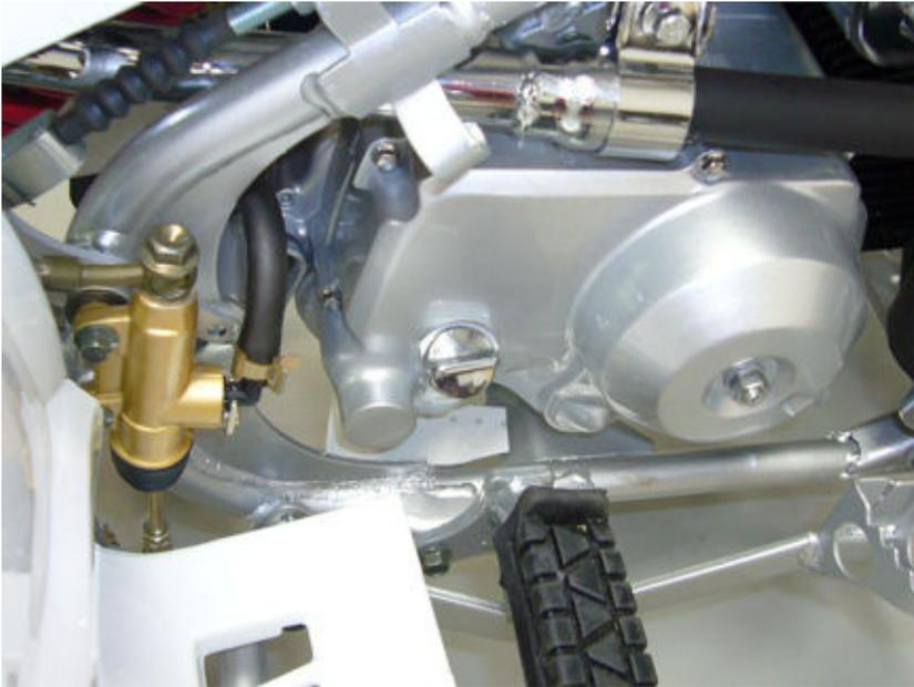
step18-fig1-Engine oil fill plug
