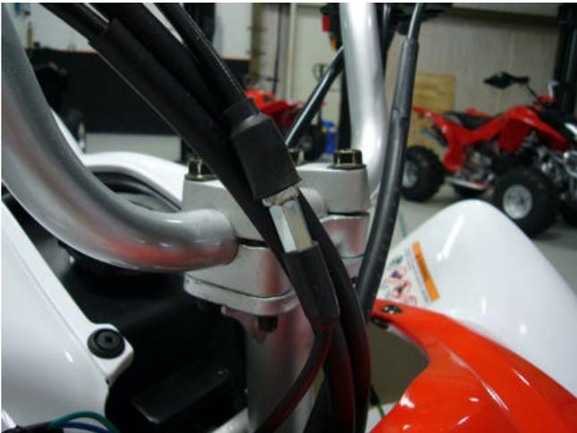
step15-fig1-Throttle cable free play adjustment
