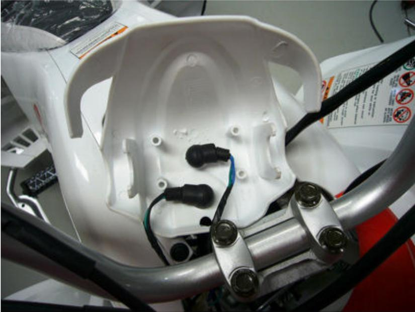
step09-fig1-Shift indicator bulbs in sockets
