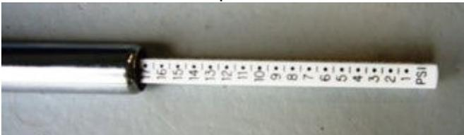
step04-fig1-Air gage with .5 pound increments
