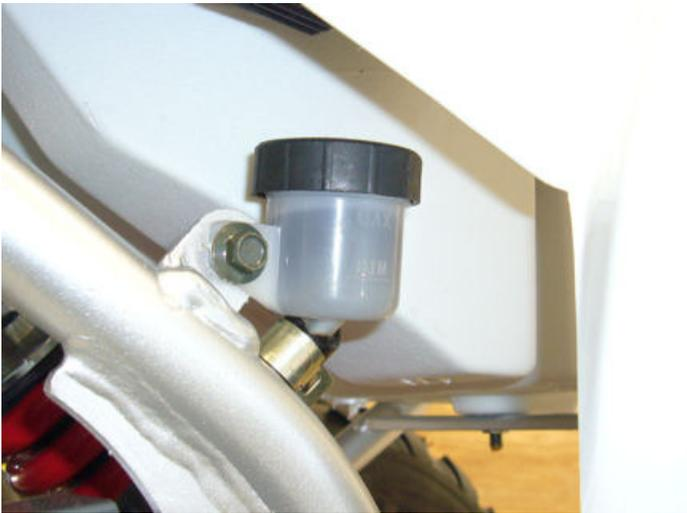
step18-fig3-Brake fluid reservoir
