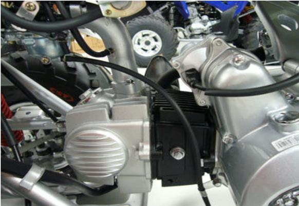
step11-fig1-Fuel drain hose routing
