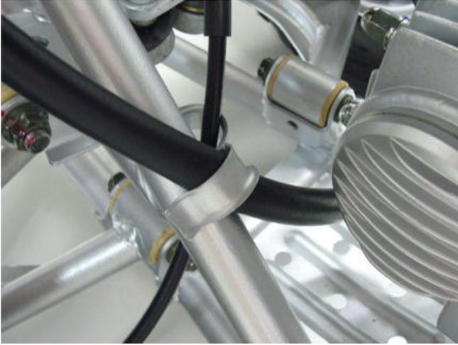
step14-fig1-Example of correct hose routing
