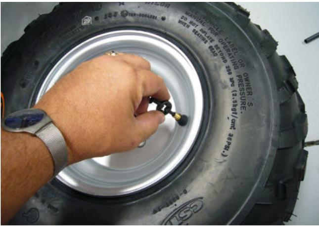
step04-fig2-Valve core tool.
