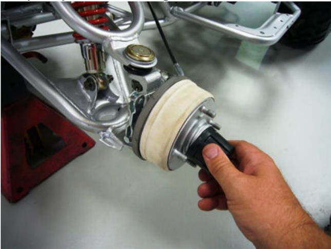
step05-fig1-Install center cap
