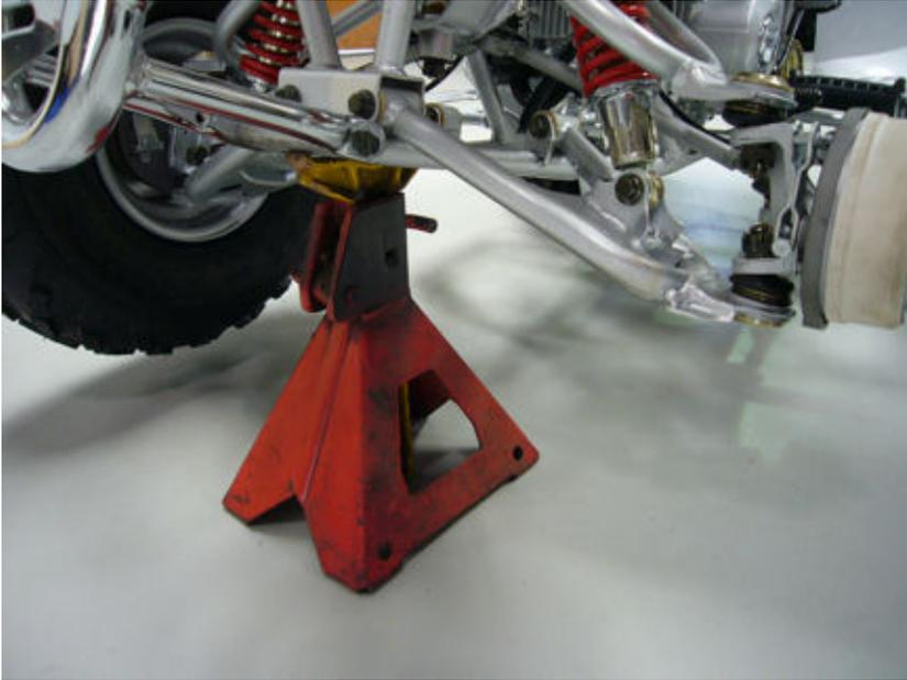
step03-fig1-Front jackstand support
