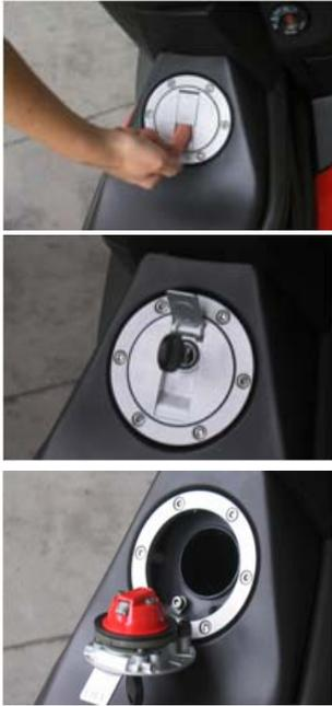
**1. Open the cover under fuel tank cap.**
