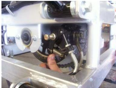
8. With a pair of needle nose pliers remove the chain.
