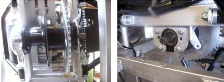
15. With an 18 mm wrench set the speedo pick up approximately 1/8” above the magnet on the differential.
