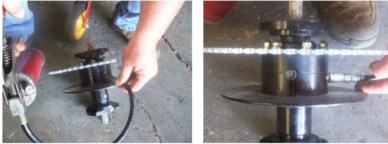
14. Install the differential with 8 – 8mm x 16 bolts and 8 – 8mm lock washers.
