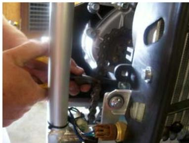
9. With a 13mm wrench remove the bolts that hold the axle bearings in place and remove the axle.
