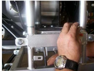
11. With an 18mm wrench loosen the speedo pickup and lift it as high as possible.
