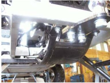
6. With an 8 and 10mm wrench remove the 250 plate.
