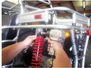
3. With 14 and 17mm wrench and remove both bolts from each knuckle, and tie up each upper A-arm.
