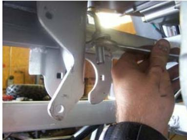
12. Using the provided template, align the square holes of it with the square holes of the bearing hanger brackets. Be sure the wider set of the 2 holes is on top.
