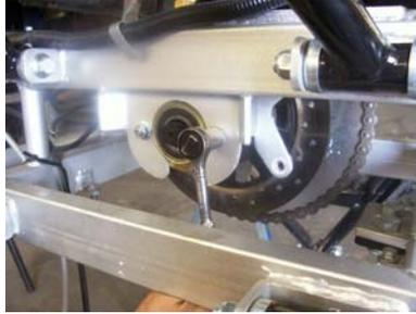
10. Loosen front and rear engine bolts.
