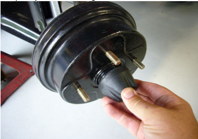
Step#05-fig#1-Center cap installation
