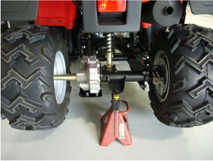
Step#06-fig#2-Rear jack support
