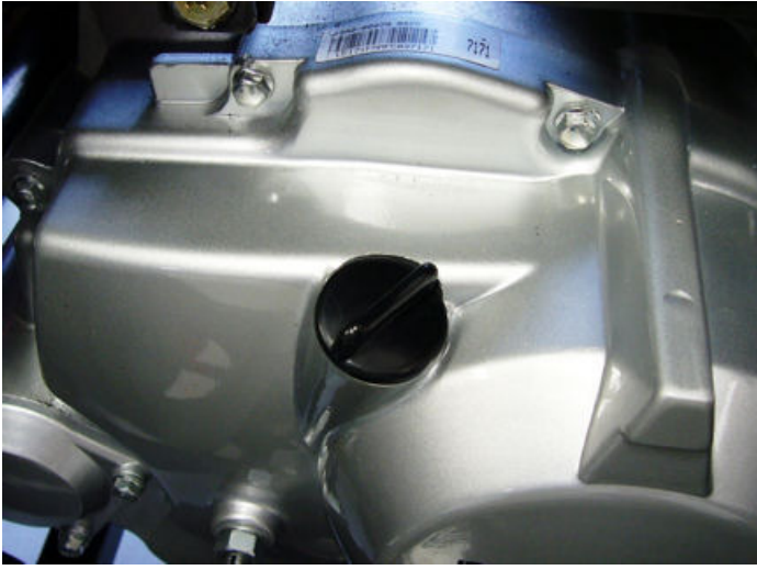
Step#19-fig#2-Inspect oil level
