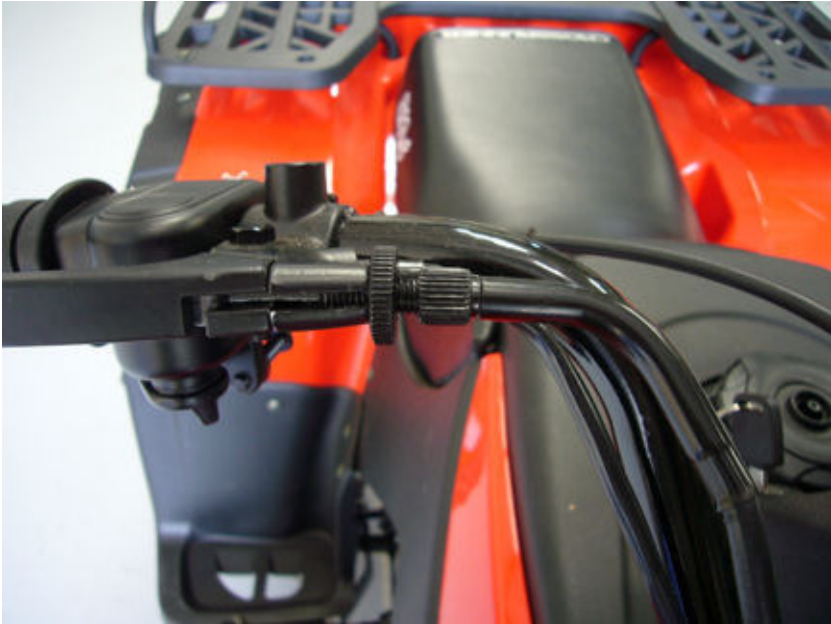
Step#16-fig#2-Front brake cable freeplay adjustment
