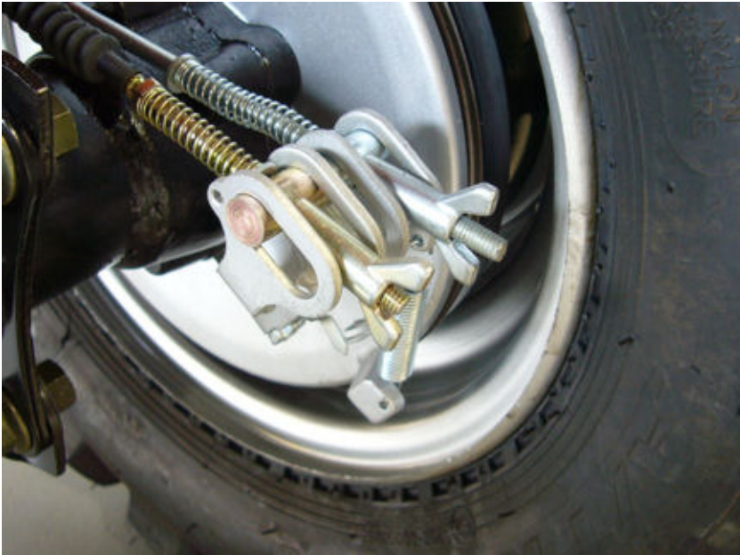
Step#16-fig#5-Rear brake adjustment
