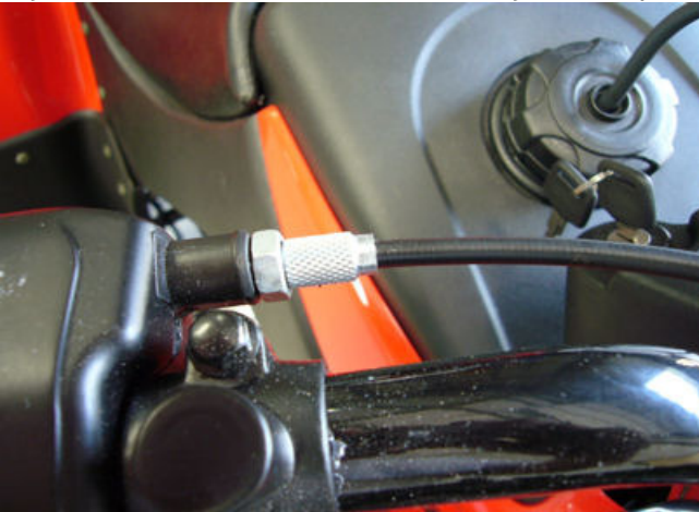
Step#16-fig#1-Throttle cable free play adjustment
