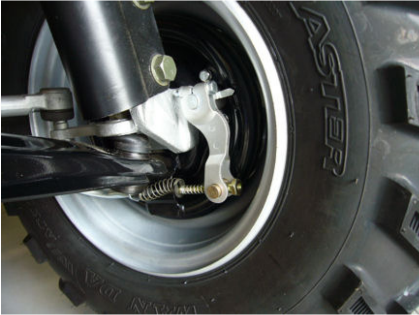
Step#16-fig#4-Front brake adjustment
