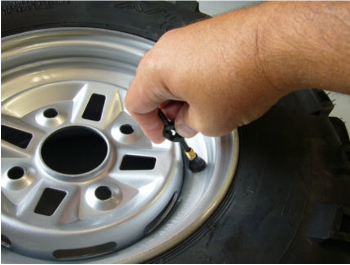
Step#04-fig#2-Valve core installation
