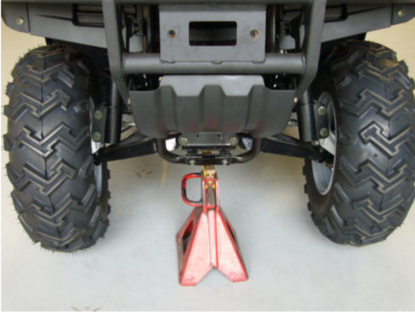
Step#03-fig#1-Front jack support
