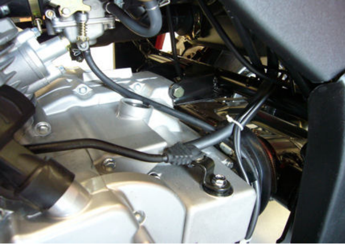
Step#15-fig#1-Inspect hose routing
