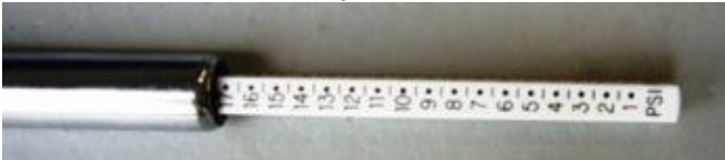
Step#04-fig#1-Air gage with .5 pound increments
