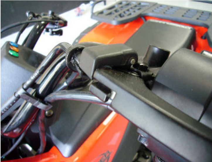
Step#06-fig#1-Set parking brake
