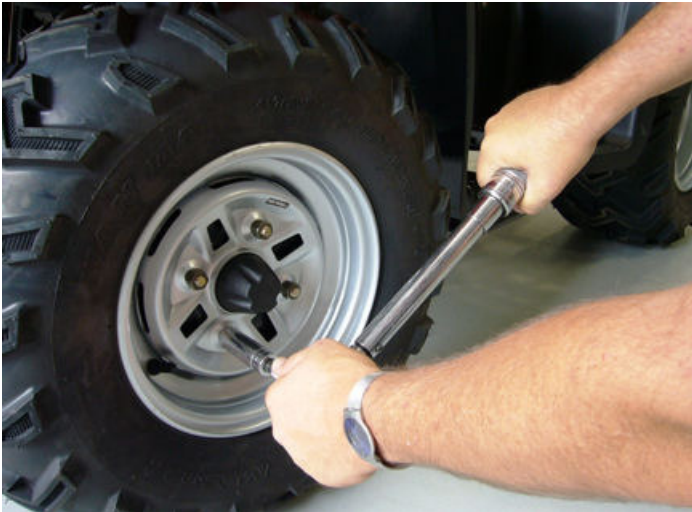
Step#07-fig#1-Torque wheels nuts
