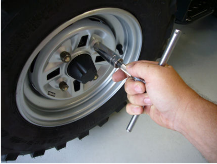
Step#05-fig#2-Hand torque lug nuts
