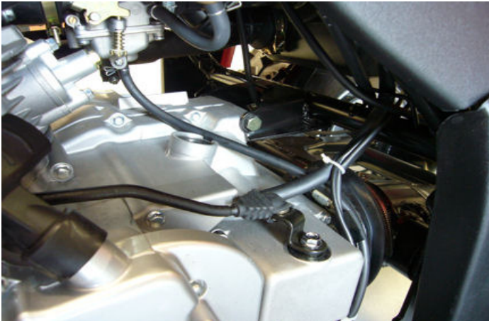
Step#12-fig#1-Fuel drain hose routing
