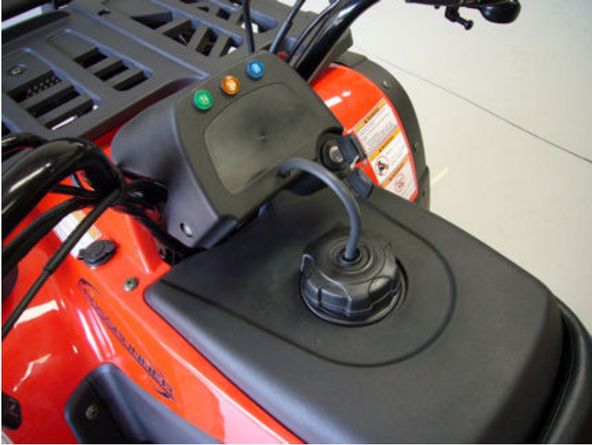
Step#19-fig#1-Fuel vent hose routing
