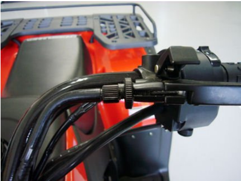
Step#16-fig#3-Rear brake cable free play adjustment
