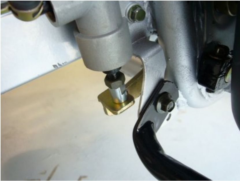
fig02-step15-Rear brake free playadjustment
