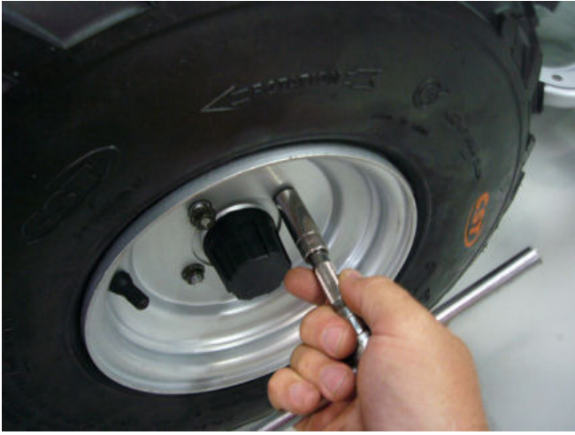
step05-fig2-Hand tighten lug nuts
