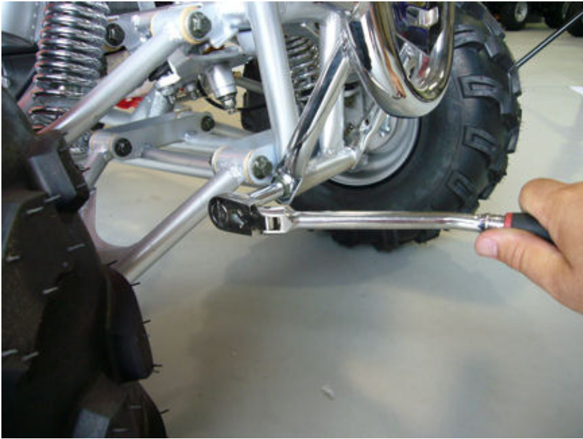
step03-fig3-Front bumper mount
