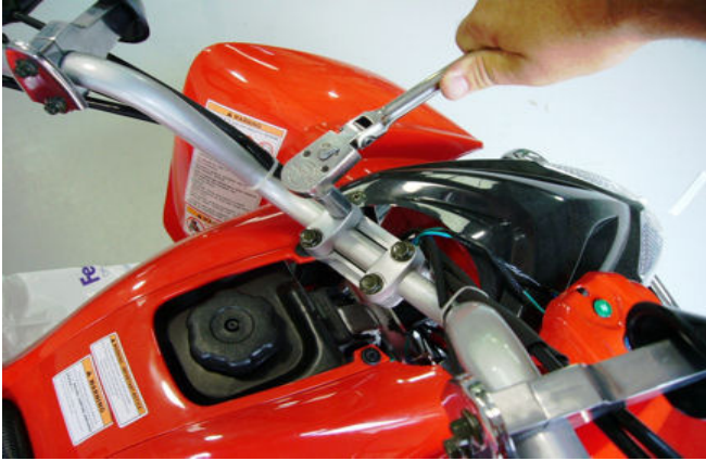
step08-fig1-Handle bar attachment
