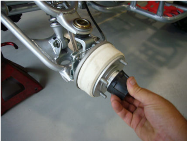
step05-fig1-Center cap installation
