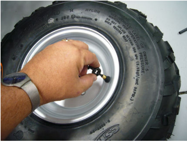
step04-fig2-Valve core tool.
