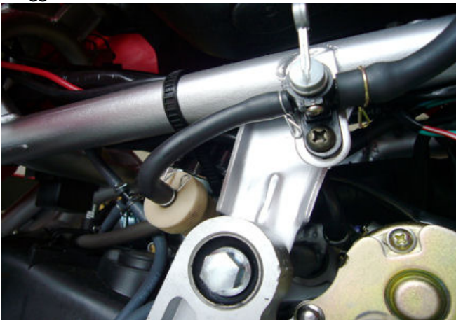
step11-fig1-Fuel line routing
