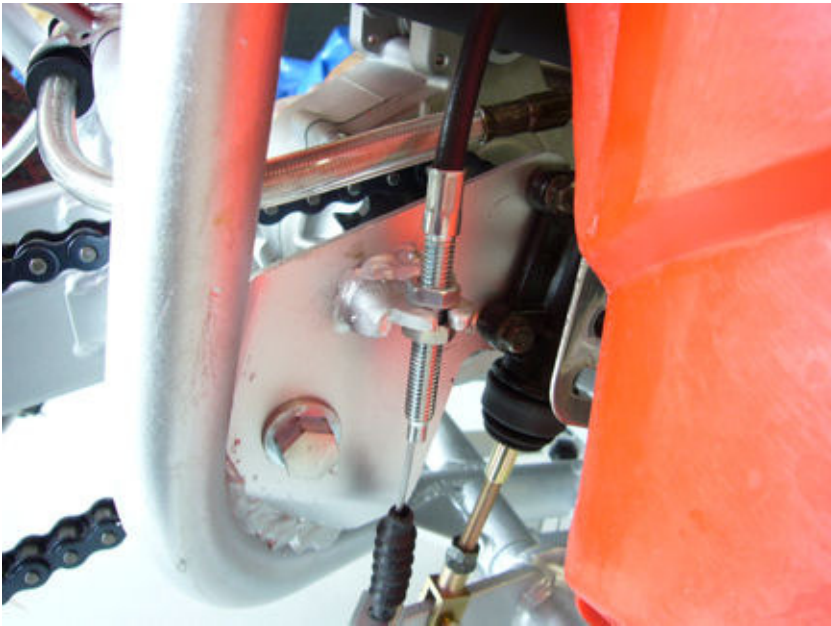
step16-fig3-Rear brake cable free play adjustment
