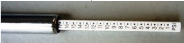
step04-fig1-Air gauge with .5 LB increments
