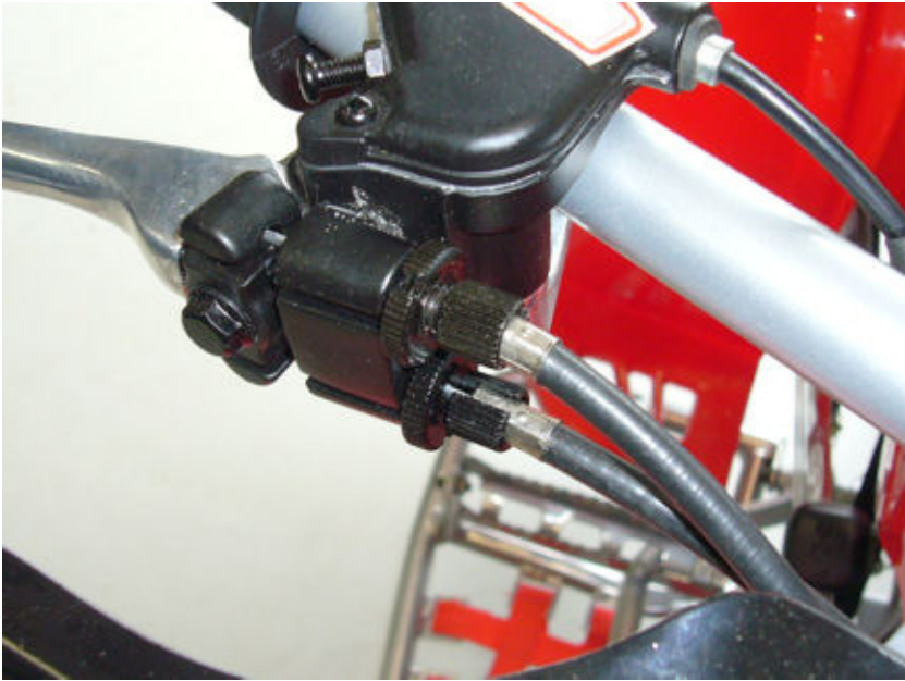
step16-fig2-Front brake cable free play adjustment
