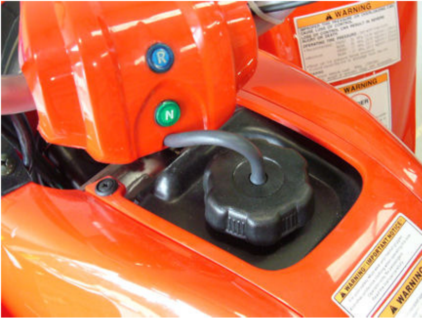
step19-fig1-Fuel cap vent tube
