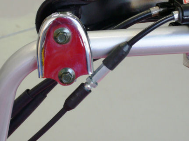
step16-fig1-Throttle cable free play adjustment
