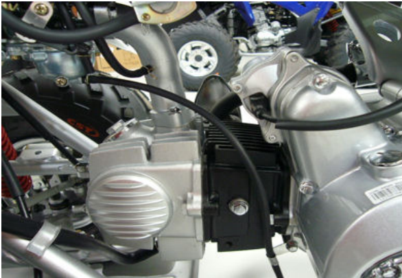
step11-fig1-Fuel drain hose routing
