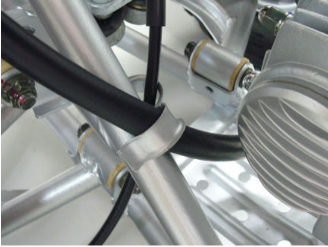
step14-fig1-Example of correct hose routing
