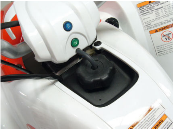
step18-fig2-Fuel cap vent hose routing
