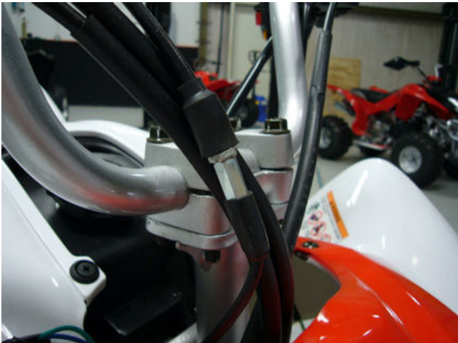
step15-fig1-Throttle cable free play adjustment
